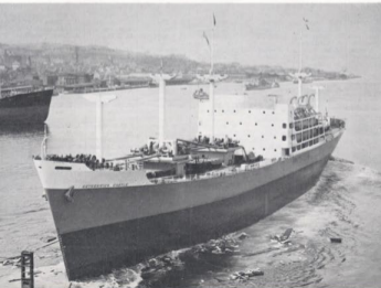
Below: The Rotherwick Castle enters the water at Greenock. She is the first refrigerated cargo ship to be built at Greenock for the Union-Castle Line
